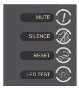
To rest the Fire Alarm Panel press 'SILENCE', 'RESET' and then 'MUTE'.
